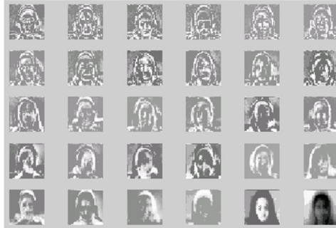
Figure 2: Eigen faces after applying Curvelet transform
